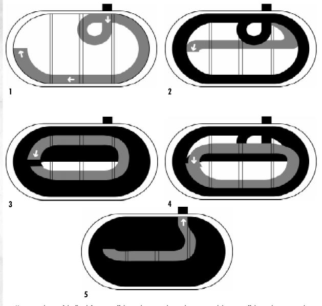
Upon completion of the flood, first turn off the wash water valve on the tower and then turn off the wash water switch on the dash. Turn off the flood water valve on the tower. Stop the auger by placing the elevator lever in the neutral position. Then raise the conditioner to the maximum position by pushing the conditioner lever to the Up position, before leaving the ice surface.
