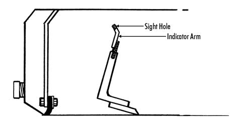
If the sight hole is filled but the blade is too high or low, go to the rear of the conditioner and using a 1 1/8" wrench, first loosen the top nut of the blade level adjusters located on each side of the rear of the conditioner shown below.
