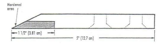
BLADE HOLDER – The blade holder is ground 1/16" higher on each end so that one shave of the ice is feathered into the adjoining shave to prevent ridges.
