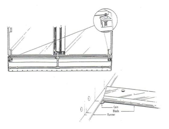
NOTE: After correct adjustment of BLADE ANGLE, with the bar covering the sight hole and the cutting edge of the blade flush with the bottom runner, raising or lowering the cutting depth will alter the bar in the sight hole. However, normal blade height adjustments do not impact blade angle and therefore no further BLADE ANGLE adjustments are necessary.
