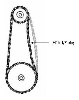
To adjust the chain tension, loosen the motor mount plate bolts and slide the motor mount until you get the proper tension, then re-tighten the motor mount plate bolts.
