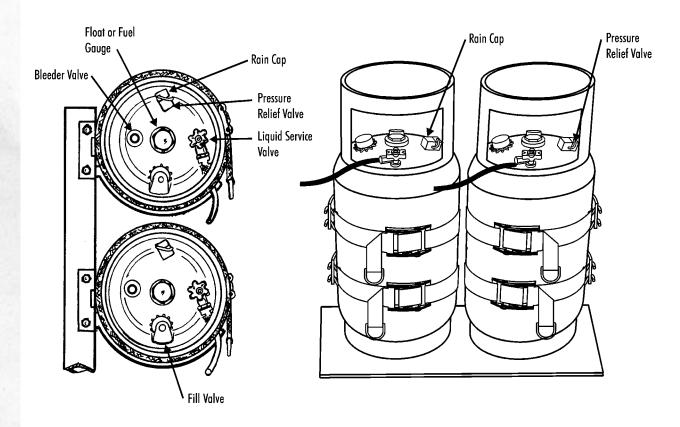
Open the service valve on both tanks and make the appropriate tank selection.
