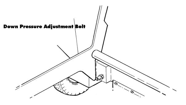
Tighten the bolts against the lift arm and lock with the jam nuts. Too much down pressure will lift the rear wheels off the ice resulting in a loss of control. Too little down pressure will result in rippled ice and gouging in the corners.
