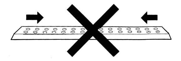
The blade holder is feathered 1/16" over the last 7" on each end. This prevents ridges forming on the ice during the resufacing operation.
