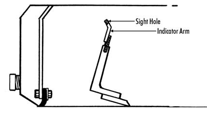
If the sight hole is filled but the blade is too high or low, go to the rear of the conditioner and using a 1 1/8" wrench, first loosen the top nut of the blade level adjusters located on each side of the rear of the conditioner shown below.
