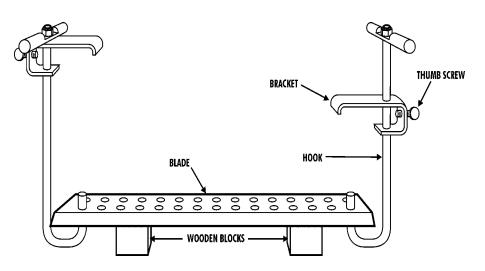
When installing a blade use the row of holes closest to the cutting edge. The second row of holes should be used when the blade has been ground down to 4" overall width.
