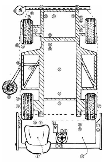
Using the drawing on the adjacent page as a guide. Make sure you grease all 25 lube points as follows:
