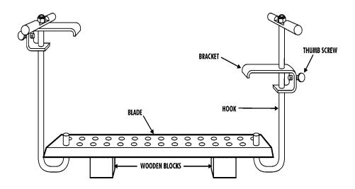
When installing a blade use the row of holes closest to the cutting edge. The second row of holes should be used when the blade has been ground down to 4" overall width.
