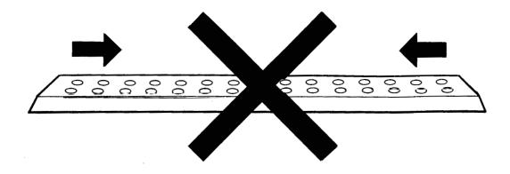
The blade holder is feathered 1/16" over the last 7" on each end. This prevents ridges forming on the ice during the resufacing operation.
