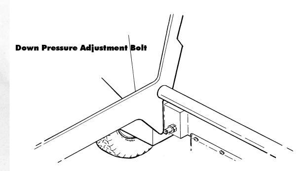
Tighten the bolts against the lift arm and lock with the jam nuts.
